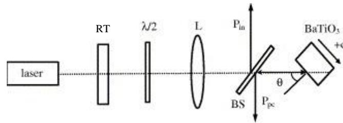
Figure 4: Experimental Setup
