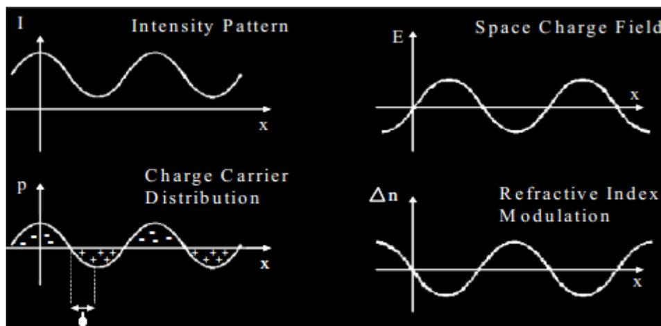
Figure 2: Photorefractive Effect
