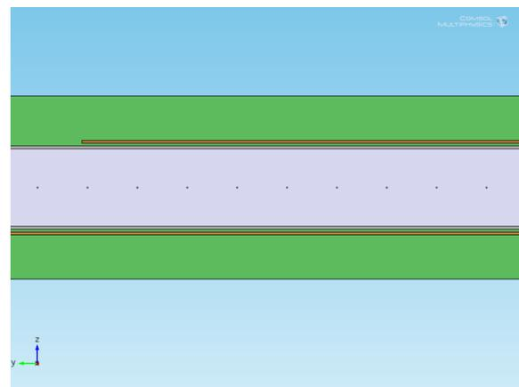
FIG. 1a. Detector's layers from top to bottom (zy plate view): pads surrounded by FR4, carbon plate (layer), wires surrounded by gas mixture, carbon plate (layer), strips surrounded by FR4 (3 layers).
