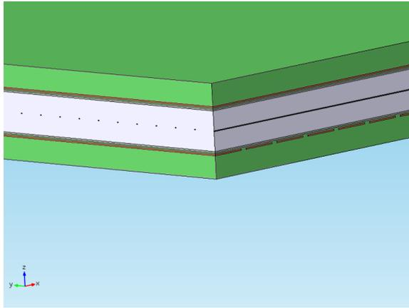
FIG. 1c. Detector's layers from top to bottom (edge cuts view): pads surrounded by FR4 (3 layers), carbon plate (layer), wires surrounded by gas mixture, carbon plate (layer), strips surrounded by FR4.
