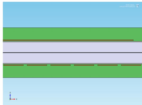
FIG. 1b. Detector's layers from top to bottom (zx plate view): pads surrounded by FR4, carbon plate (layer), wires surrounded by gas mixture (3 layers), carbon plate (layer), strips surrounded by FR4.
