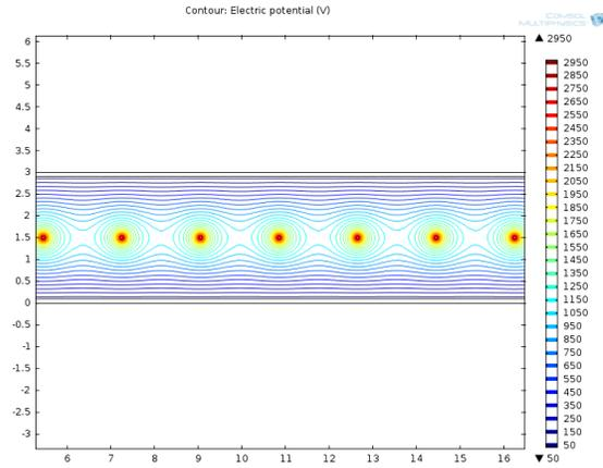
FIG. 2a. The electric potential between the carbon plates with no charge distribution in the medium (contour lines view).
