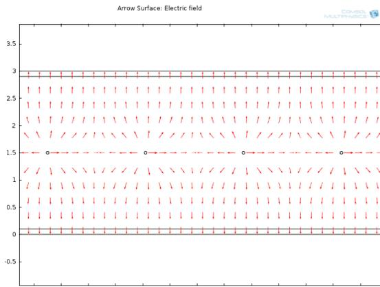
FIG. 3b. The electric field between the carbon plates with no charge distribution in the medium (logarithmic arrows – shows direction and the relative field's size at each point).
