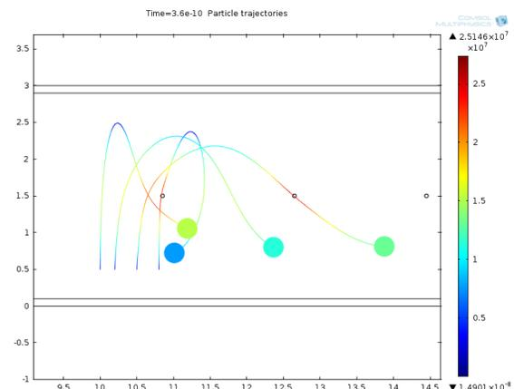
FIG. 6b. The electrons' motion from 0.5[mm] at y axis.
