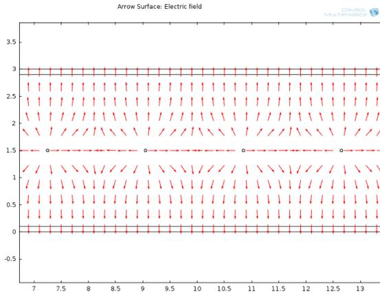
FIG. 3a. The electric field between the carbon plates with no charge distribution in the medium (normalized arrows – shows only direction of the field, which actually is also the positively charged particles motion's direction).
