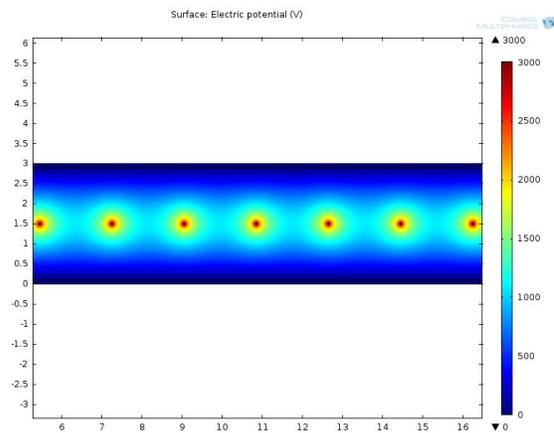
FIG. 2b. The electric potential between the carbon plates with no charge distribution in the medium (continuous domains view).
