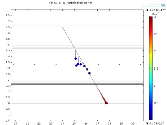
FIG. 4. The red particle is the muon, which crossed the gas medium, while the rest of the particles (the blues) are the electrons emitted from the ionized  $\text{CO}_2$  gas.
