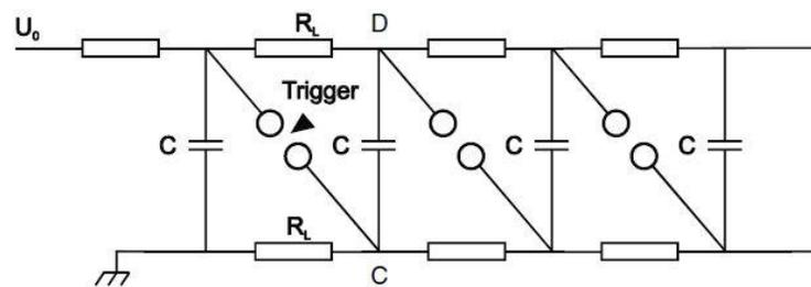
Figure 5: *Marx generator circuit with unipolar charging through the resistors  $R_L$*
