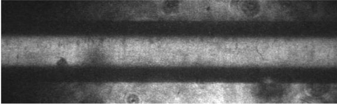
Figure 1: *Typical image of the self-light emission from the surface of the discharge channel and shadow image of expanding shock wave in water*
