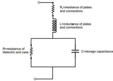
Figure 3: *Lumped circuit model of a capacitor*
