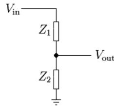
Figure 8: *Simple active voltage divider circuit scheme*
