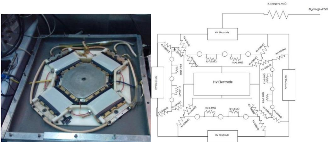
Figure 4: *from left to right – The microsecond timescale generator. The microsecond timescale generator circuit scheme*
