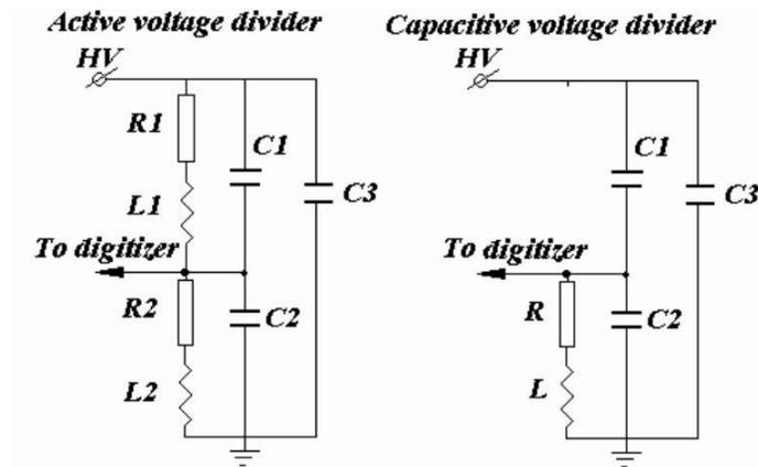
Figure 9: Active and Capacitive voltage dividers circuit schemes
