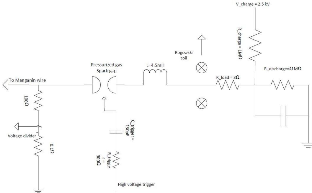
Figure 6: *The measuring circuit scheme*
