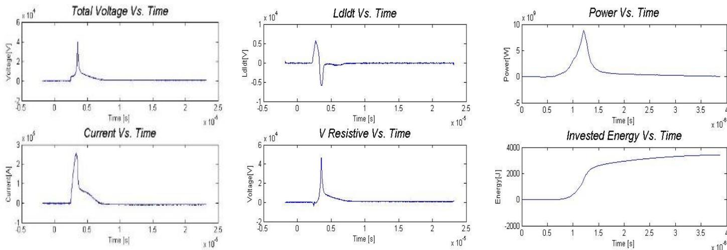
Figure 11: from left to right: Typical waveforms of the current and total voltage of the microsecond timescale generator. Typical inductive voltage and resistive voltage of the microsecond generator with the wire array. The Power and the energy invested in the experiment.
